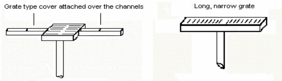
Figure 2. Alternate Drain Configurations
