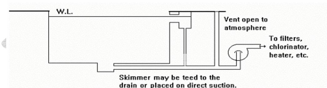
**Figure 4. Vent System to relieve Main Drain Suction**
