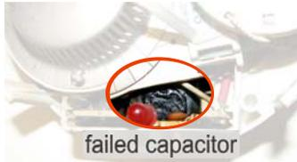
Figure 2. Failed capacitor
