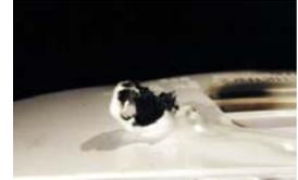
Figure 8. Capacitor shell lodged in the housing
