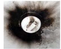
Figure 5. Soot ring around the alarm
